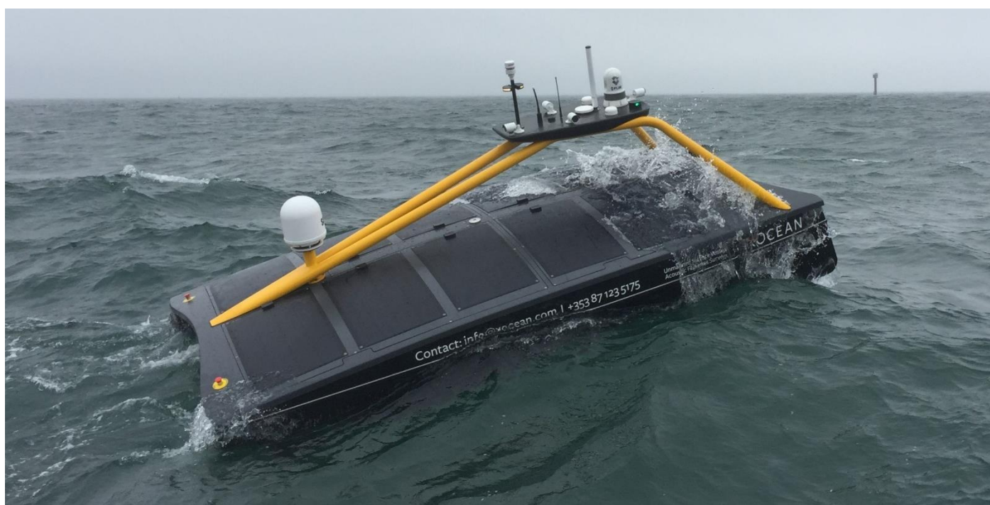
FIGURE 2: XOCEAN'S XO-450 UNCREWED SURFACE VESSEL (USV)
