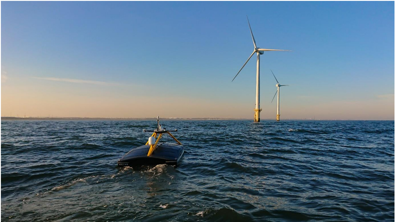
FIGURE 8: XOCEAN'S XO-450 UNCREWED SURFACE VESSEL (USV)
